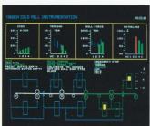
Now decide how the dynamic information should be presented. This is done interactively, in the form of fields, defined for numerical values, curves, schematic and flow diagrams, thermometers, histograms, etc.
