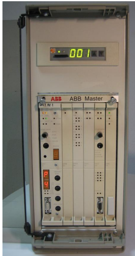
Figure 1 The DDR unit of type NDDD 002 mounted in a MasterView 830 cabinet.
